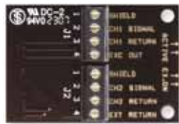
U30 Built in Analog Input Port (2 inputs) VIA
